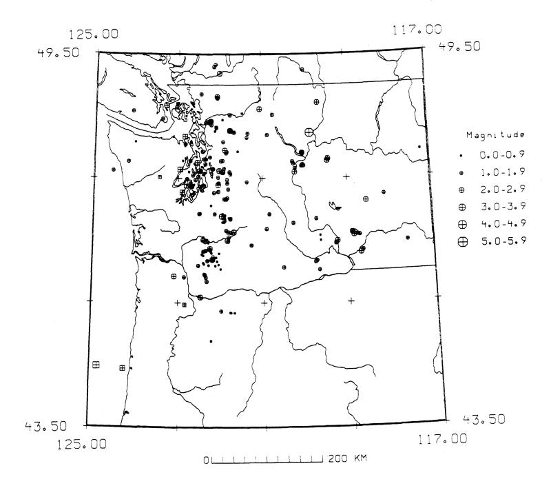
Figure 3. Earthquakes located in Washington and northern Oregon with magnitudes greater than 0.0, first quarter 1989. A square symbol indicates that an event located with a depth greater than or equal to 30 km. Octagonal symbols are used for events shallower than 30 km.
